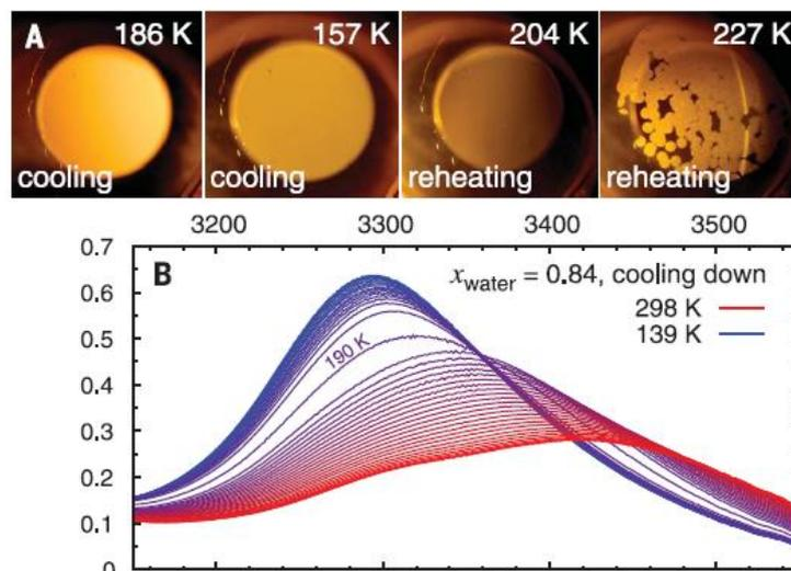
*Optical observation of the solutions and infrared spectra recorded during cooling [5].*
