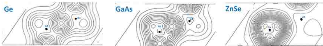
Figure 2.5: DFT calculation of the sum of the valence band electron distribution in between two atoms of Germanium (diamond structure), GaAs and ZnSe (zinc blend structure). In germanium the totally symmetric electron charge distribution with a higher concentration in the line relying the two atoms is the sign of the covalent bond. We observe a progressively more ionic character in GaAs (III-V) and ZnSe (II-VI) which translates in the asymmetric electronic distribution.
