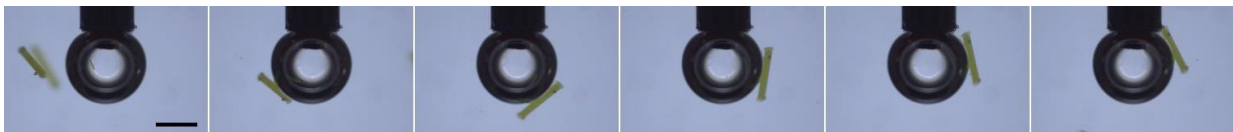
Figure 2 Image sequence of a preliminary experiment performed at ILM. We observe the adsorption of a single polymer fibre (time lapse 0.4 s, scale bar 1 mm).
